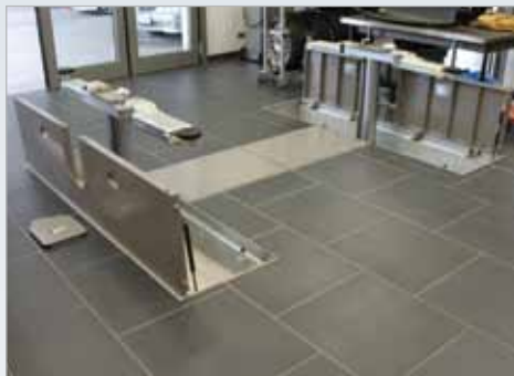
A pneumatic damper system assists the opening and closing of the cover
