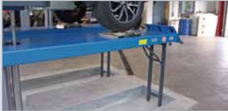
Height levelling for 1200 mm using axle measurement supports. Telescopic axle measurement supports up to 1700 mm (optional).
