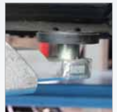
The support plate of the swivel arm support can be positioned very exactly at the relevant support points under the vehicle.
