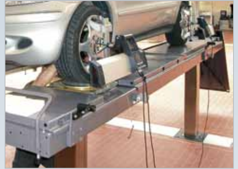
High degree of accuracy as an axle measurement lifting device.
