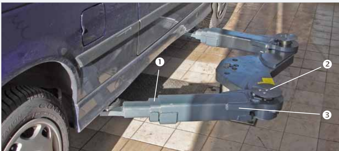
Swivel arm system with very large support area.
