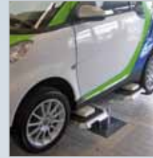
Shortened flat support, e.g. for Smart 1150 – 1750 mm.
