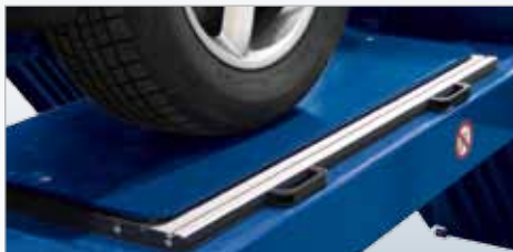
Precision sliding plate Minimum breakaway torque 5 Nm an minimum displacement force 15 N for 500 kg wheel load, large amount of steel balls, hardened running surface, collection grooves for dirty water.
