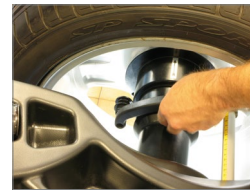
Auto distance and diameter measurement.
