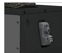
Supports house measuring heads and recharge batteries.
