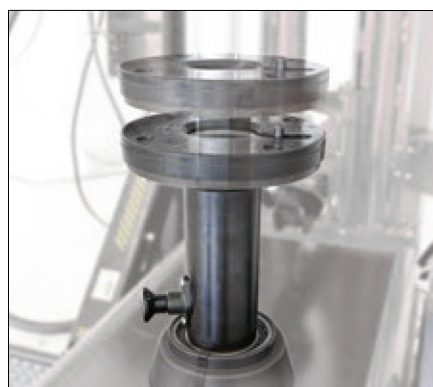
Extra-grip clamping device. Three adjustable working heights.
