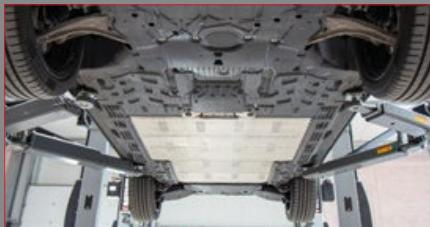
The depth of the outer arm and lifting adaptor are equal, thus, reducing the possibility of the arm making contact with the vehicle underbody.
