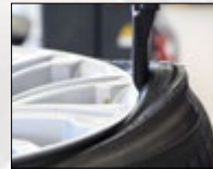
Patented tool in plastic anti-scratch material.
